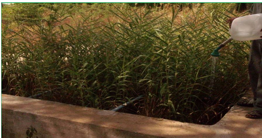
Figure 3: Charging of Nickel Solution or EDTA into the Constructed Wetland System
