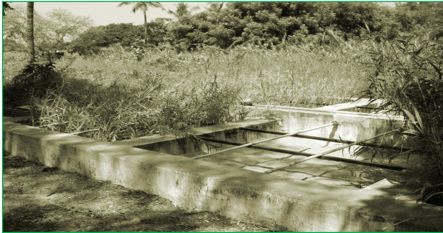
Figure 1: Pilot Scale Constructed Wetland System (Vertical Flow) at Anna University, Chennai-India
